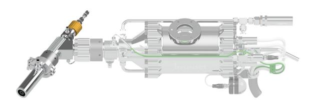
The Central Injector Kit is an accessorie for the Impact Gun. It enables a central powder injection into the convergent section of the laval nozzle. The optimized injection reduces the risk of powder adhesion for very fine and particularly temperature-sensitive powders, which increases the cost-effectiveness of the process. Depending on the requirements, the position of the powder injector can be changed mechanically.
