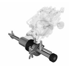
The Cooled Powder Injector is an accessorie part for the Central Injector Kit. It is connected to the Central Injector Kit and cools the injector tube with compressed air. This is useful for soft materials, which tend to stick to the injector. This assembly can be customized to individual length.
