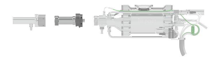
The Prechamber Extension Kit is an accessorie for the Impact Gun and is used to extend the distance between the powder injection and the smallest cross-section of the laval nozzle. This component has a direct influence on the residence time of the powder in the high temperature area of the Impact Gun. As a result, the single powder particles can absorb more heat and can be deformed easier when they hit the surface.
