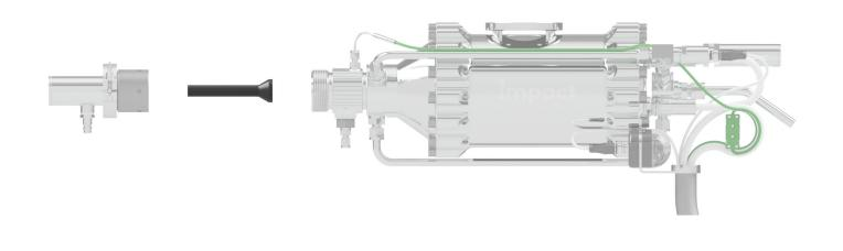
The nozzle Injector - OUT2 is a shortened nozzle with a higher expansion rate. Operation in conjunction with air or water cooling is recommended. This greatly reduces wear and tear and the risk of nozzle clogging.
