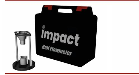
The Hall Flowmeter Kit (DIN EN ISO 4490) can ascertain the flowability of a powder quickly and precisely by determining the mobility of the powder particles in relation to each other. The measured value is expressed by the time required for 50 grams of metal powder to flow through a calibrated funnel. The Hall Flowmeter Kit is stored in a suitcase that includes:
