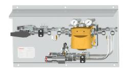
The Gas Supply Control Panel - He is a pressure reducing unit which can connect any helium gas supply system to the Impact-EC-GM-Unit EvoCSII. The component is designed for the control of a maximum inlet pressure of up to 200 bar. The pressure control includes a dome pressure reducer and ensures stable process
