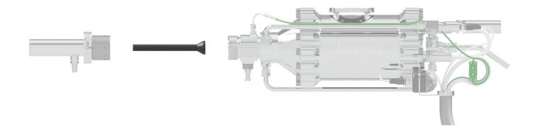
The nozzle Injector - OUT1 is an universal nozzle for all types of powders. Operation in conjunction with air or water cooling is recommended. This greatly reduces wear and tear and the risk of nozzle clogging.
