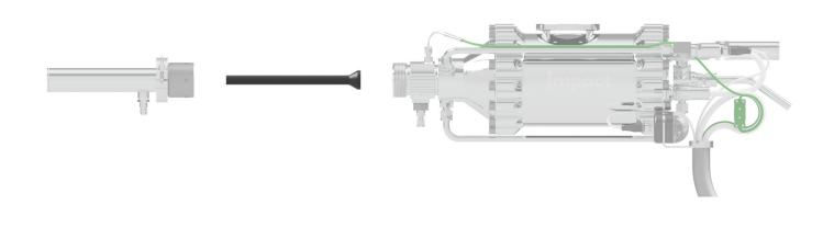
The nozzle Injector - OUT4 is an extended nozzle, especially for higher particle speeds. Operation in conjunction with air or water cooling is recommended. This greatly reduces wear and tear and the risk of nozzle clogging. The nozzle Injector - OUT4 is compatible with all versions of the Impact Gun. It can also be used in combination with various accessories. The WC - nozzle has a high wear resistance and is suitable for very hard materials.
