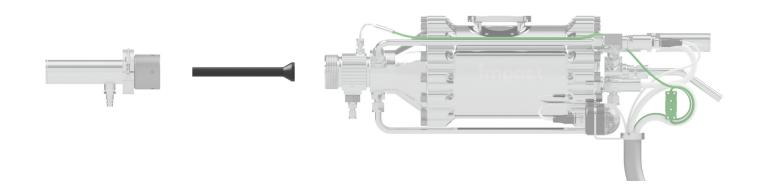
The nozzle Injector - OUT5 is a nozzle that is specially designed for the use of helium as process gas. Thanks to the smaller nozzle throat, the helium consumption is up to 30% lower and higher process parameters can be reached. Operation in conjunction with air or water cooling is recommended. This greatly reduces wear and tear and the risk of nozzle clogging.
