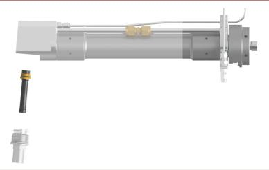
The nozzle Injector - IN2 is designed for the ID Coating Device and is suitable for bores with a minimum diameter of Ø107 mm. Due to the length of the nozzle, a high particle velocity is reached.
