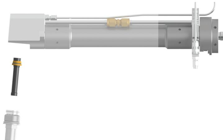
The nozzle Injector - IN2 is designed for the ID Coating Device and is suitable for bores with a minimum diameter of  $\varnothing 107$  mm. Due to the length of the nozzle, a high particle velocity is reached.
