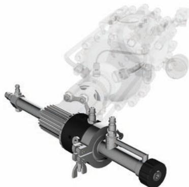
The Cooled Powder Injector is an accessory part for the Central Injector Kit. It is connected to the Central Injector Kit and cools the injector tube with compressed air. This is useful for soft materials, which tend to stick to the injector. This assembly can be customized to individual length.
