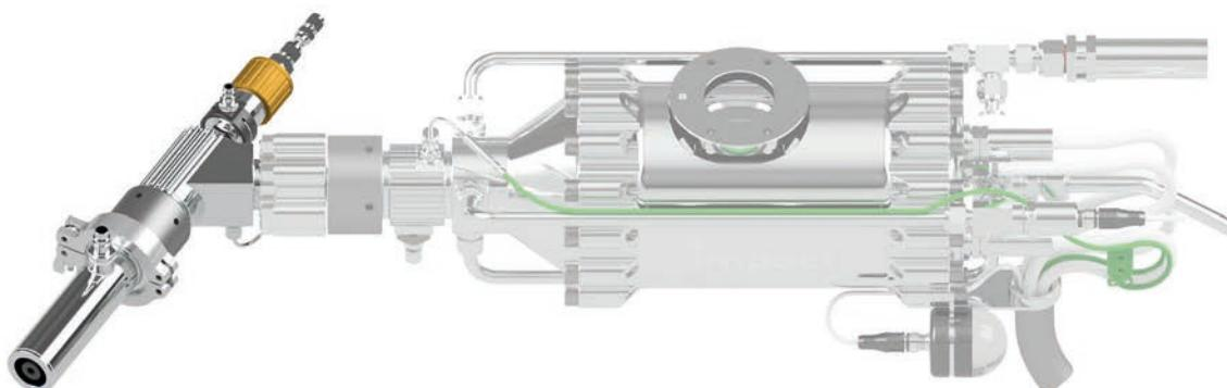
The Central Injector Kit is an accessory for the Impact Gun. It enables a central powder injection into the convergent section of the laval nozzle. The optimized injection reduces the risk of powder adhesion for very fine and particularly temperature-sensitive powders, which increases the cost-effectiveness of the process. Depending on the requirements, the position of the powder injector can be changed mechanically.
