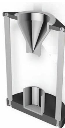
The Hall Flowmeter Kit (DIN EN ISO 4490) can ascertain the flowability of a powder quickly and precisely by determining the mobility of the powder particles in relation to each other. The measured value is expressed by the time required for 50 grams of metal powder to flow through a calibrated funnel.
