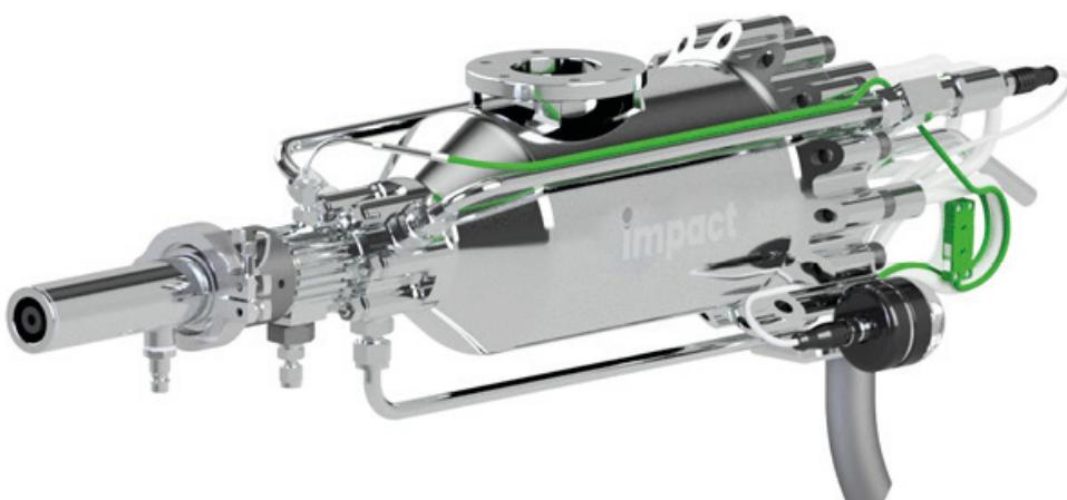
The Impact Gun 5/8 EvoCSII can reach a pressure of 50 bar and a process temperature of up to 800 °C. This makes it ideal for processing easily deformable materials. Due to the compact and lightweight design, it is also possible to coat components that are difficult to access. It is also equipped with an operating hours counter to enable conclusions to be drawn about the duration of use.
