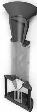
The Scott Volumeter Kit is designed to determine apparent density of the different powders as per DIN ISO 3923. Due to the different apparent density small deviations in particle size and structure can be detected. The results of the measurements help to find out the powder feed rates.
