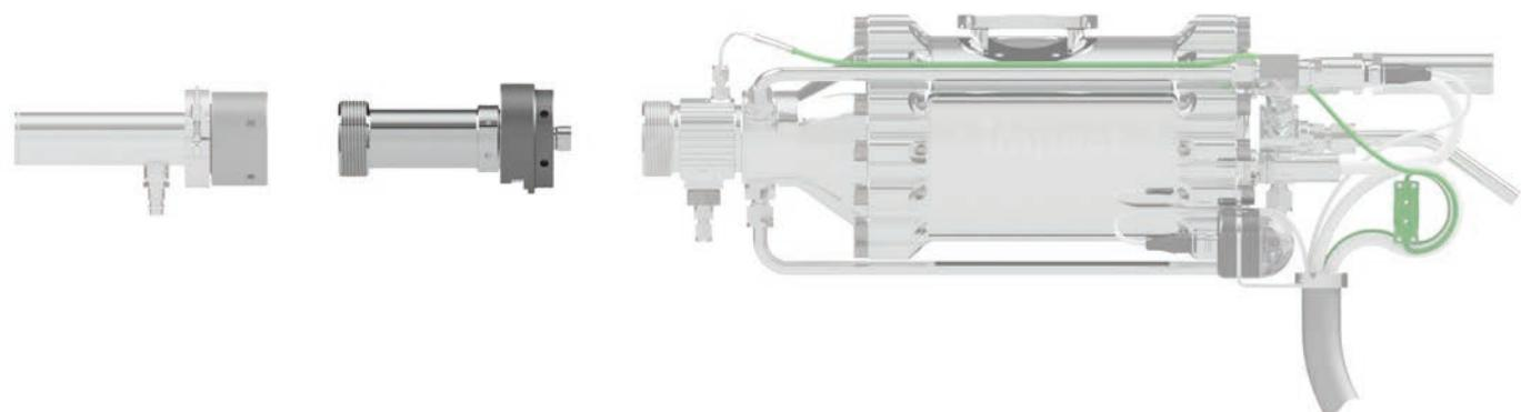
The Prechamber Extension Kit is an accessory for the Impact Gun and is used to extend the distance between the powder injection and the smallest cross-section of the laval nozzle. This component has a direct influence on the residence time of the powder in the high temperature area of the Impact Gun. As a result, the single powder particles can absorb more
