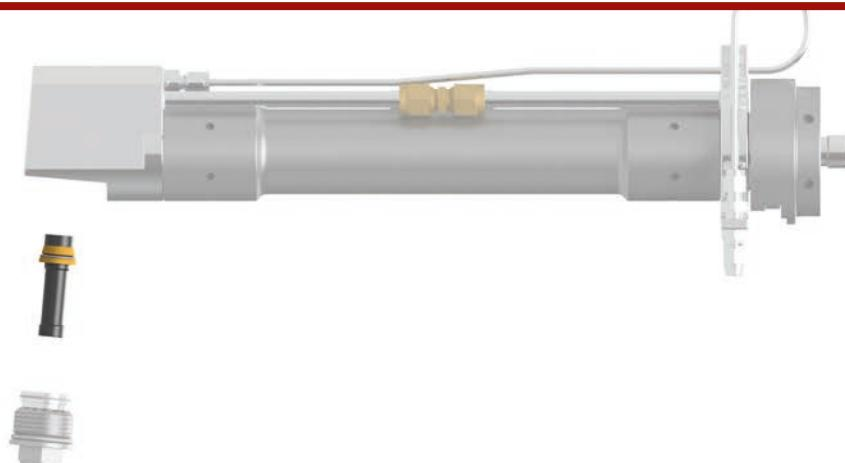
The nozzle Injector - IN3 is designed for the ID Coating Device and is suitable for bores with a minimum diameter of Ø84 mm. Operation is only possible in conjunction with water cooling. This greatly reduces wear and tear and the risk of nozzle clogging.
