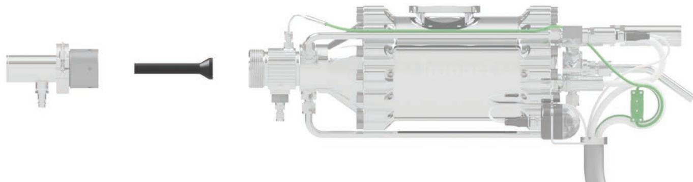
The nozzle Injector - OUT2 is a shortened nozzle with a higher expansion rate. Operation in conjunction with air or water cooling is recommended. This greatly reduces wear and tear and the risk of nozzle clogging.
