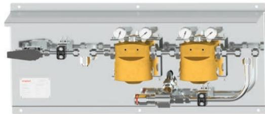
The Gas Supply Control Panel - N2 is a pressure reducing unit which can connect any nitrogen gas supply system to the Impact-EC-GM-Unit EvoCSII. The component is designed for the control of a maximum inlet pressure of up to 200 bar. The two-stage pressure control includes two dome pressure reducer and ensures
