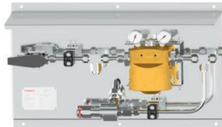
The Gas Supply Control Panel - He is a pressure reducing unit which can connect any helium gas supply system to the Impact-EC-GM-Unit EvoCSII. The component is designed for the control of a maximum inlet pressure of up to 200 bar. The pressure control includes a dome pressure reducer and ensures stable process
