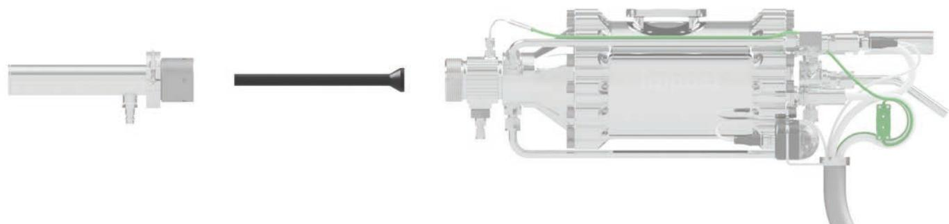
The nozzle Injector - OUT4 is an extended nozzle, especially for higher particle speeds. Operation in conjunction with air or water cooling is recommended. This greatly reduces wear and tear and the risk of nozzle clogging. The nozzle Injector - OUT4 is compatible with all versions of the Impact Gun. It can also be used in combination with various accessories.
